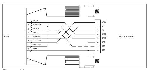
Figure 14: AT Computer Adapter
